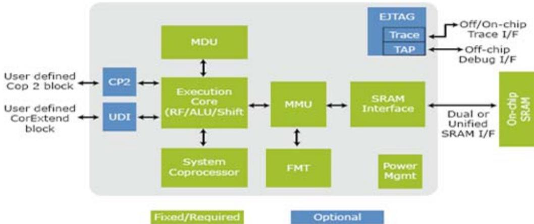
To reduce gate count, the M4K core provides a comprehensive set of build time configuration options. Configurable options include enabling/disabling debug features, setting the number and type of debug/trace breakpoints, enabling fast or slow MDU, setting the number of GPR files and enabling either unified or separate data and address SRAM interface.
