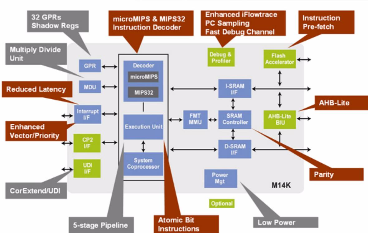
The M14K core has all of the same advantages that the M4K core has over the Cortex-M3: higher performance, lower power, smaller size, more configurability and flexibility. In addition, the M14K core provides additional benefits over the Cortex-M series as shown in [Table 2](#).
