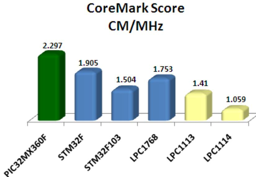
The M4K-based PIC32, executing with 2 wait state memory, achieves a higher CoreMark/MHz than competitive Cortex-M3 and Cortex-M0 based devices operating with 0 wait state memory. Fig 4 shows a PIC32 outperforms Cortex-M3 STM and NXP solutions (in blue) at equivalent clock frequencies by 20-50%, Cortex-M0 NXP solutions (in yellow) by over 63%.
